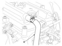
c. Loosen the valve cover bolts and then remove the cover(A). (next page)
