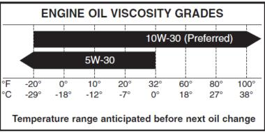
Temperature/Engine Oil Viscosity
