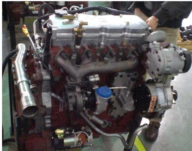
Exhaust side of 4H engine
