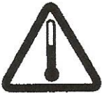
Hot surface warning
