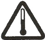
Hot surface warning
